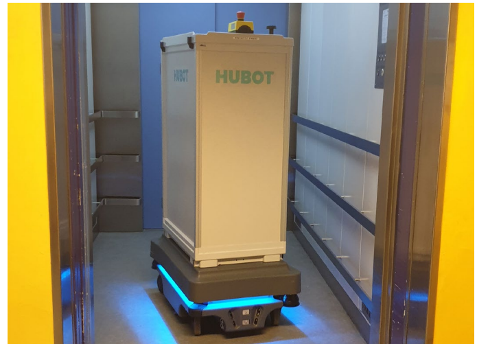
MiR200 AMR autonomously riding an elevator, using RealSense depth cameras for navigation between floors.
