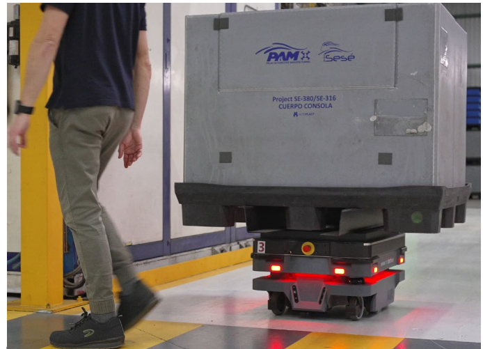
MiR250 AMR navigating safely around people using RealSense depth cameras for obstacle detection.
