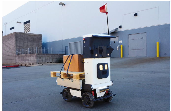
Cartken Hauler robot equipped with RealSense sensors, enabling safe navigation in outdoor environments.
